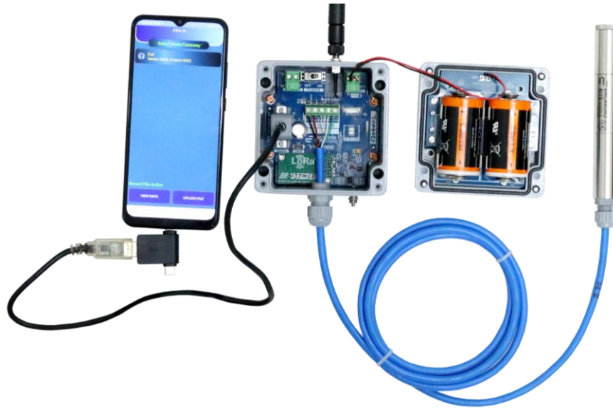
Figure 6-6 EWN-01V VW node connected to Android phone with FTDI cable via OTG adaptor
