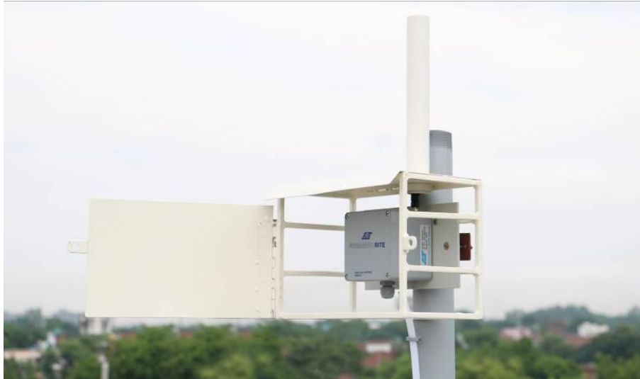
Figure 9-2 EWN-01V VW node mounted on mast with a protection box (antennae inside protective tube)
